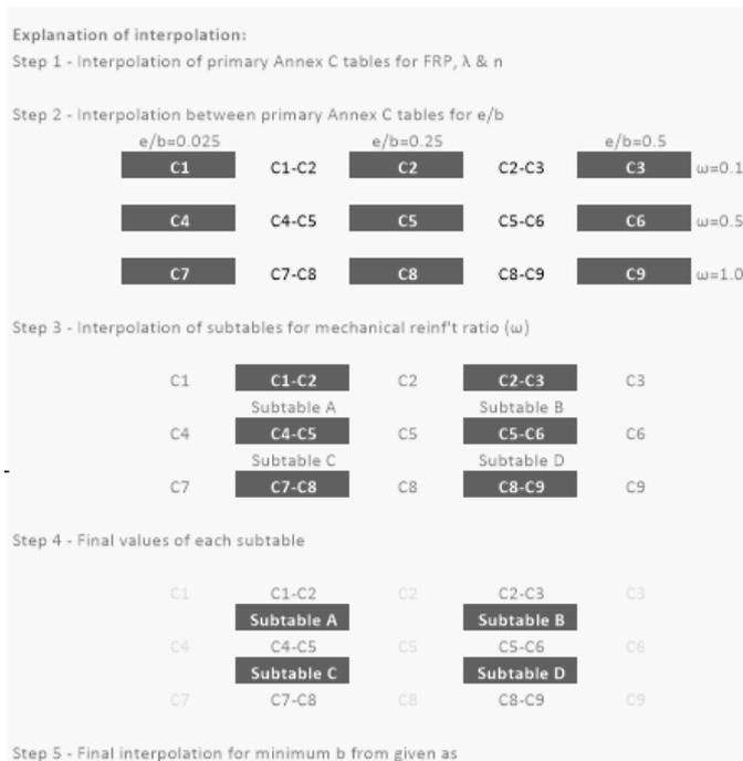
If two values are given at the end of the interpolations, the spreadsheet will determine the minimum dimension based on the value of the design axis distance. If the axis distance is larger than the greater axis distance of the outputs, the larger of the output values will be selected. If the axis distance is less than the minimum in the outputs no value will be given.
