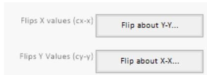
Figure 7 - Flip axis buttons
